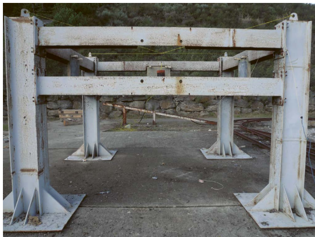
Figure 4. Test bench used in the blast tests.
