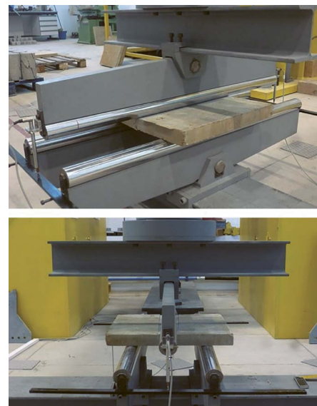
Figure 12. Experimental setup for the tests of the residual strength of the slabs.
