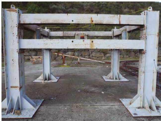
Figure 4. Test bench used in the blast tests.
