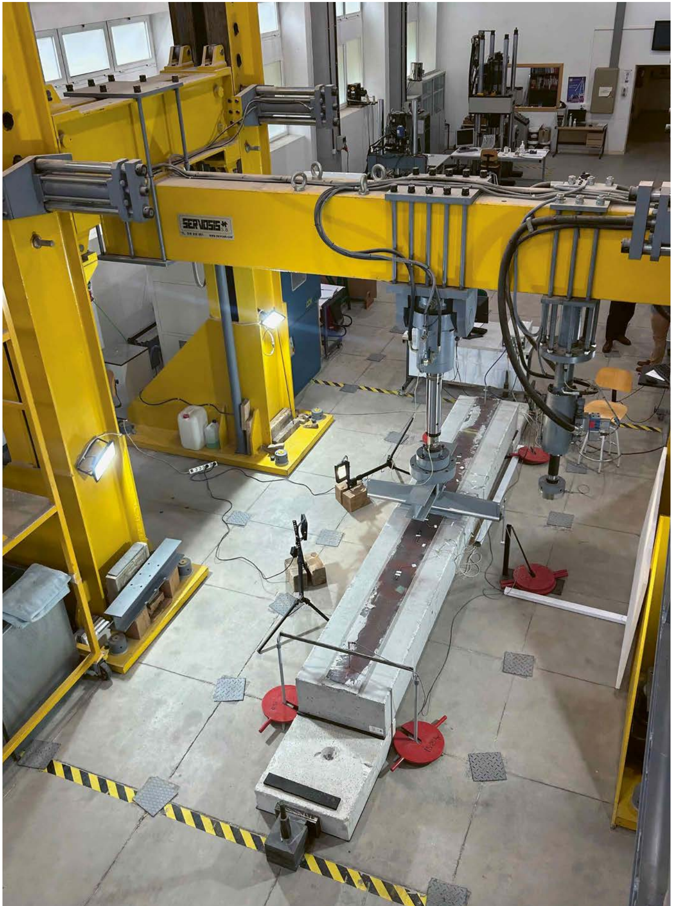
Figure 2: Beam being tested in hogging configuration.
