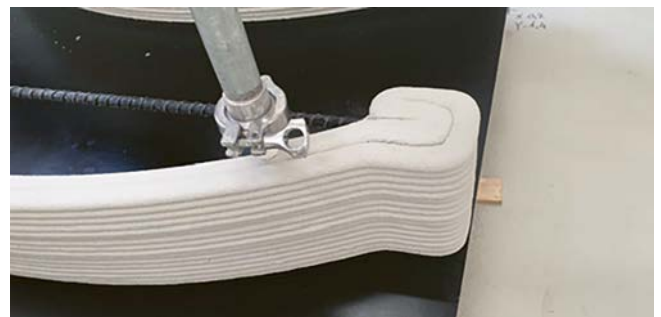
Figure 4. Anchorage details of 3D concrete printed shell element including tensile FRP reinforcement during the 3D concrete printing process (Lab. of Construction Materials and Technologies, BME, Budapest) (Photo GL Balázs).
