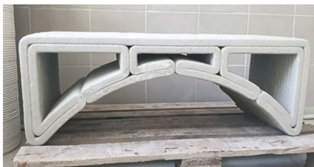
Figure 3. Arch bridge produced in 3D concrete printing (Lab. of Construction Materials and Technologies, BME, Budapest) (Photo GL Balázs).
