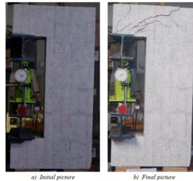
Figure 2. Specimen  $\phi 20$ -c10-B-1L-b before and after the test.
