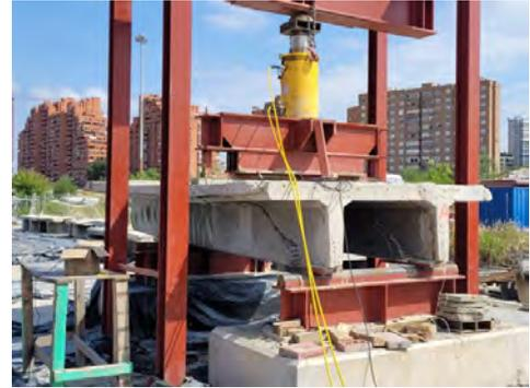
Figure 2. Full-scale shear test on prefabricated prestressed beams to update the uncertainties of the resistance model.
