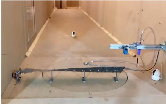
Figure 1. Torsional instability of the solar tracker.
