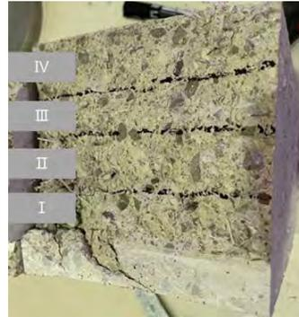
Figure 2. Fracture surface of a prismatic specimen (RA-9)
