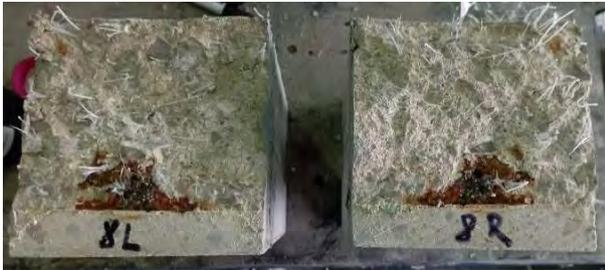
Figure 1. Typical cross section of a corroded beam (pre-cracked and exposed).
