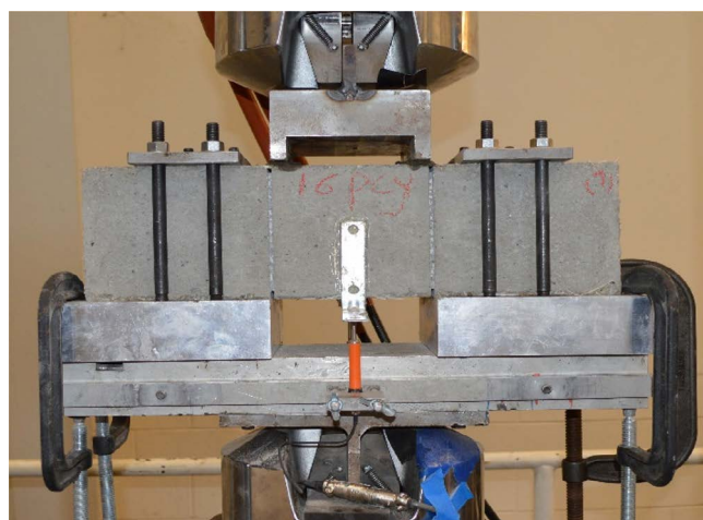
Figure 4. Test setup for direct shear tests performed by Mostafazadeh et al. [12,13].
