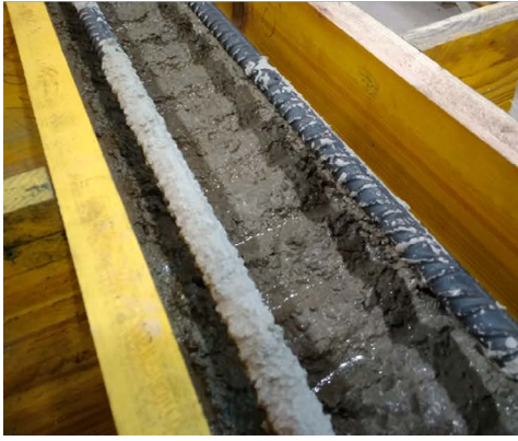
Figure 4. Pictures of the concrete surface before pouring the concrete of the slab: (a) “Very rough” surface; (b) “Smooth” surface.
