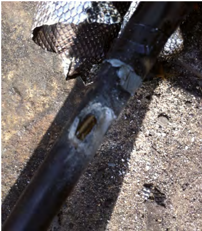
Figure 11. Internal aspect of strand and protective coating, the opening was made to assess the current state of the wires.
