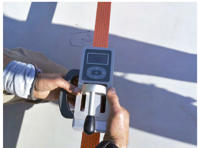
Figure 15. Ratched belts under 5kN tension every meter. Checking of the force. Credit: Pfeifer Seil- und Hebeteknik GmbH.
