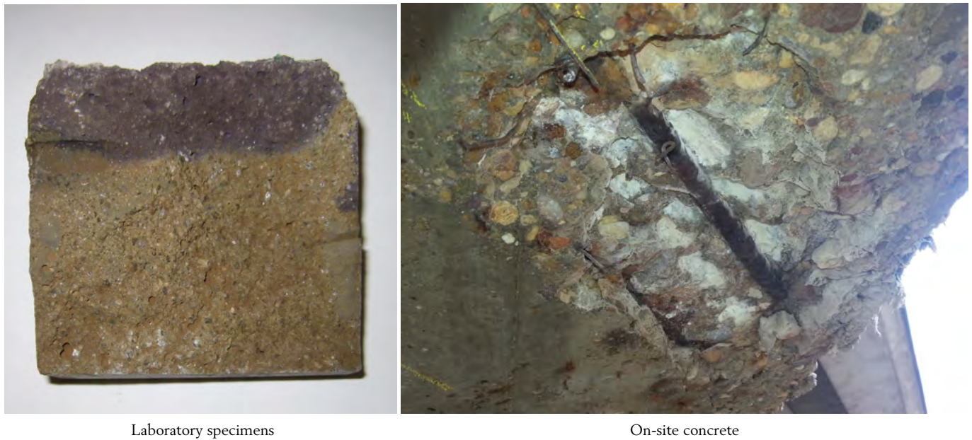
Figure 21. Colour-based silver nitrate indicator chloride test on concrete.
