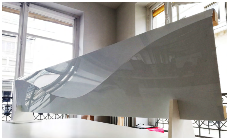
Figure 13. Pictures of the prototype. The finish is very smooth and the reflections highlight the double-curvature of the panel.
