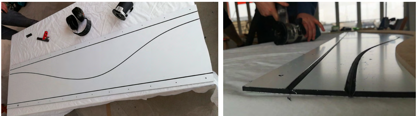
Figure 12. Machining of the composite sheet to generate both straight and curved folds.
