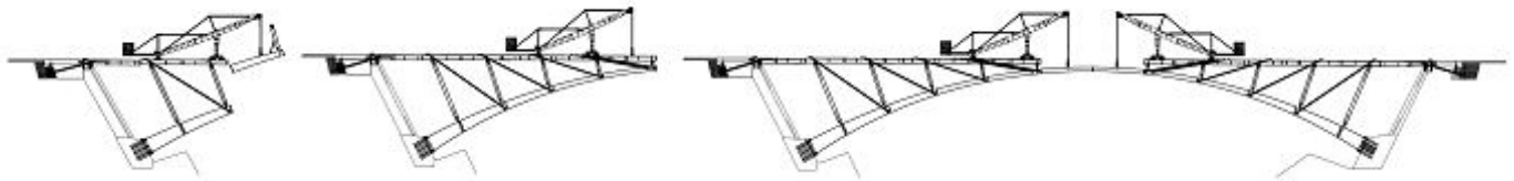
Figure 27. Erection stages of the steel structure.
