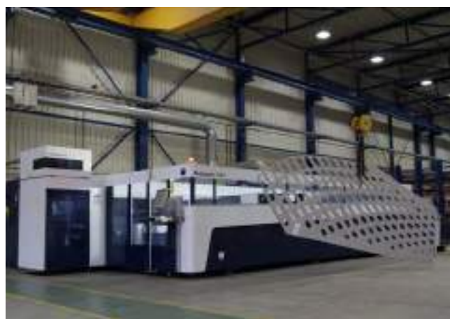
Figure 12. Laser cut plate in front of the laser cutter. ©Outokompu
