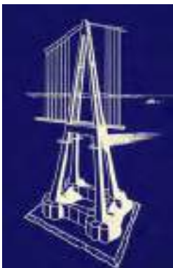
Figure 18. Off shore type bridge pier concept for 300 m water depth.
