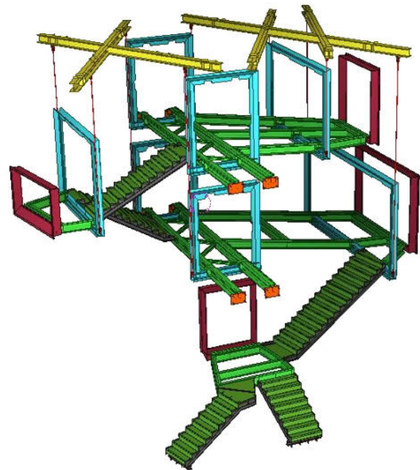
Figure 18. View of the Tekla model developed for fabricating the steel structure.
