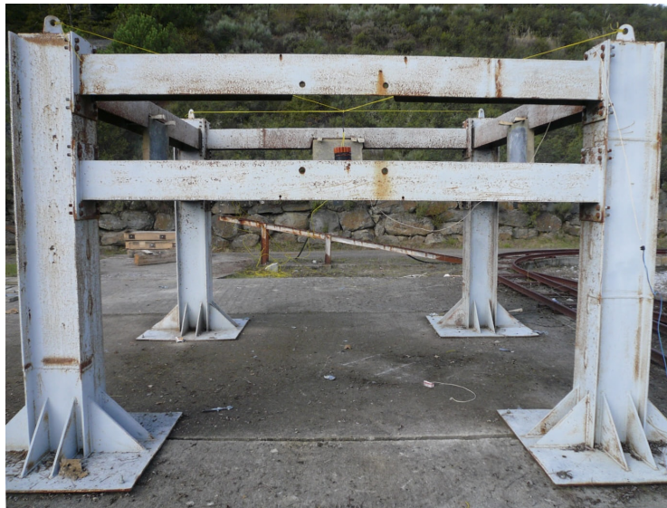
Figure 4: Test bench used in the blast tests.
