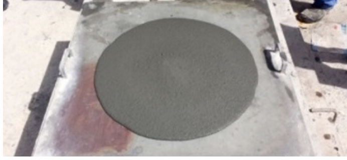
Figure 1: Slump flow test.
