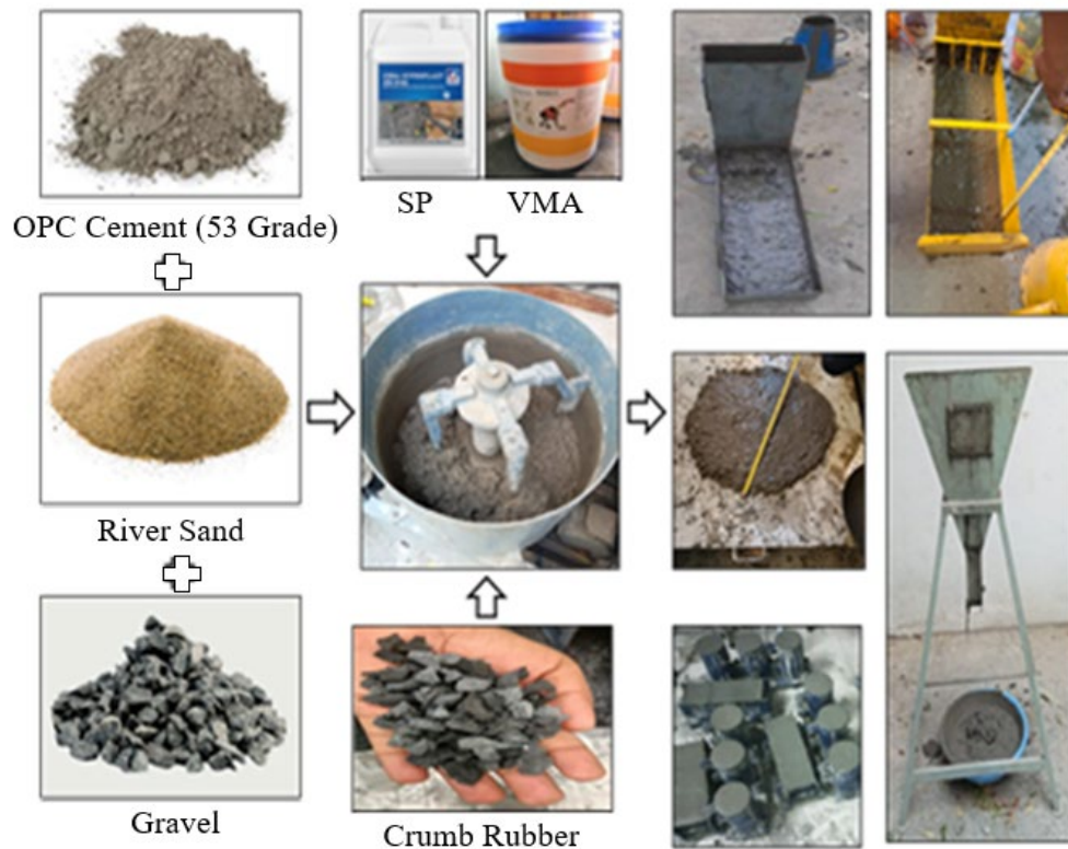
Figure 2: Experimental procedure: mixing, casting, and fresh-state testing (slump flow and L-box) of SCC mixtures
