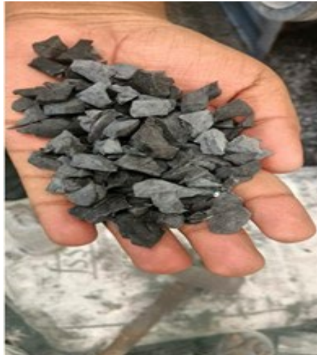
Figure 1: CR derived from waste tires, used as a sustainable partial replacement for natural coarse aggregate in SCC mixes
