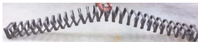
Figure 9. Helical CFCM reinforcement.
