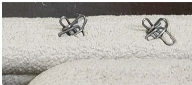
Figure 6. Increase of interlaminar shear in 3D printed concrete by STAREX elements (Lab. of Construction Materials and Technologies, BME, Budapest) (Photo GL Balázs).
