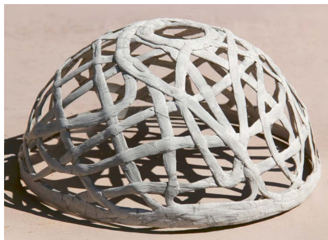
Figure 8. Spherical shell model in CFCM reinforcement [14].
