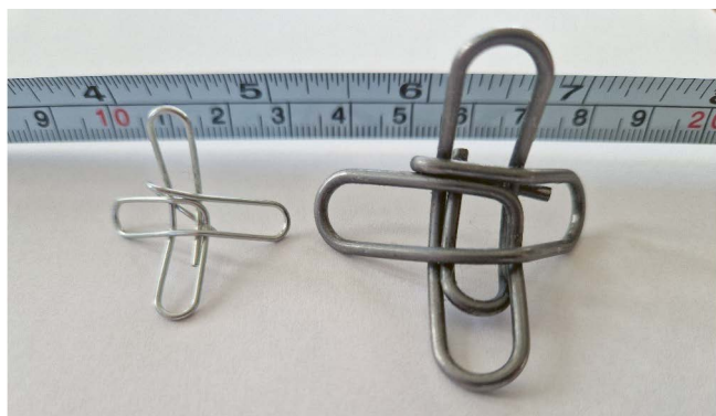
Figure 7. STAREX reinforcing elements of different sizes (Lab. of Construction Materials and Technologies, BME, Budapest) (Photo GL Balázs).
