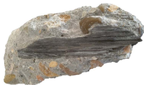
Figure 10. Bond layer of an embedded CFCM reinforcement opened after failure of the element – is still entirely connected to the concrete Lab. of Construction Materials and Technologies, BME, Budapest) [14] (Photo GL Balázs).
