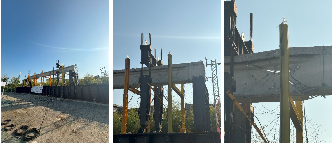
Figure 12. Failure mechanism of the PC bridge deck beam with top RC slab under four-point loading with shear span ratio \alpha \approx 0.32 .
