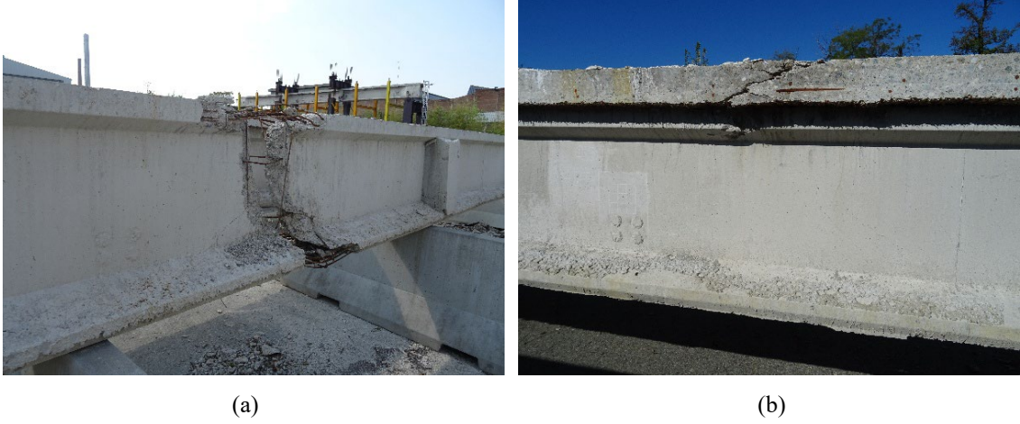
Figure 5. Failure mechanism after the full-scale load test based on three-point loading with shear span ratio \alpha \approx 1.00 of PC bridge deck beam (a) without top RC slab and (b) with top RC slab.
