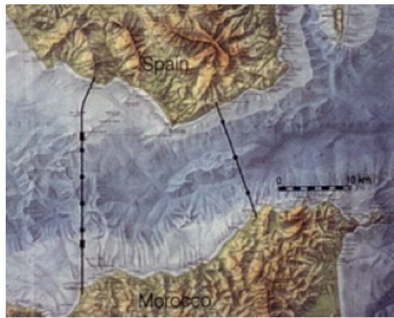
Figure 17. Gibraltar Strait - 3 x 3500 m suspension bridge solution.
